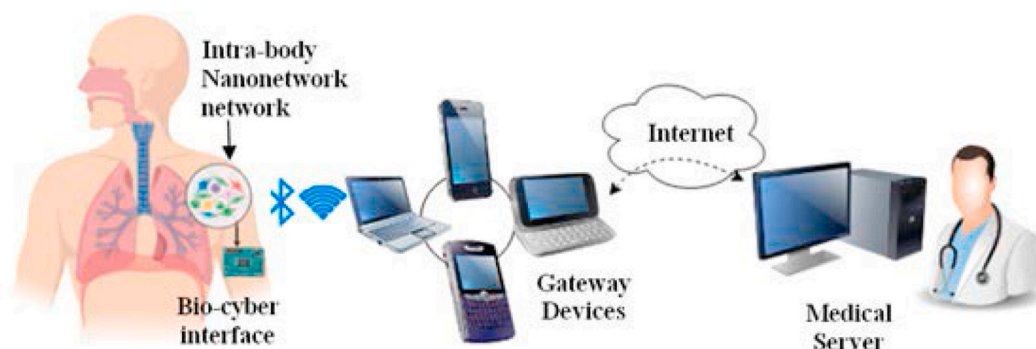
Fig. 1. Internet of Bio nano things architecture where inbody bio chemical signals and sensory data is relayed through bio cyber interface through Internet to Medical server for further processing.
