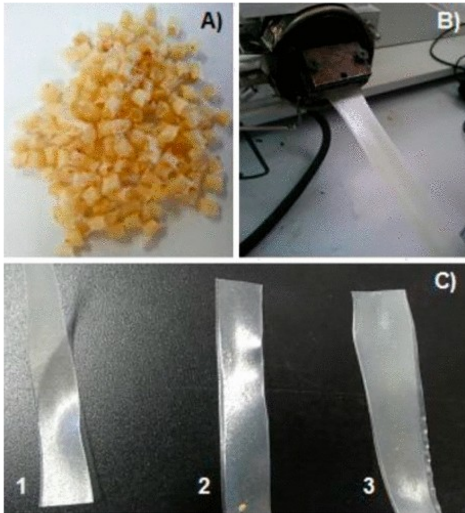
Fig. 5. Compound chitosan granules and extrusion machine to create the packaging film (Wang, H.; Qian, J.; Ding, F. 2018)
