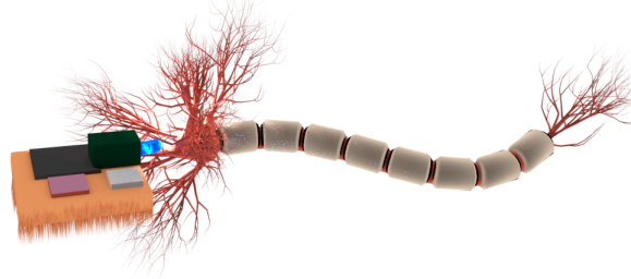
Figure 2: Illustration of a WiOptND that interfaces to an engineered neuron that is sensitive to light at a specific wavelength.
