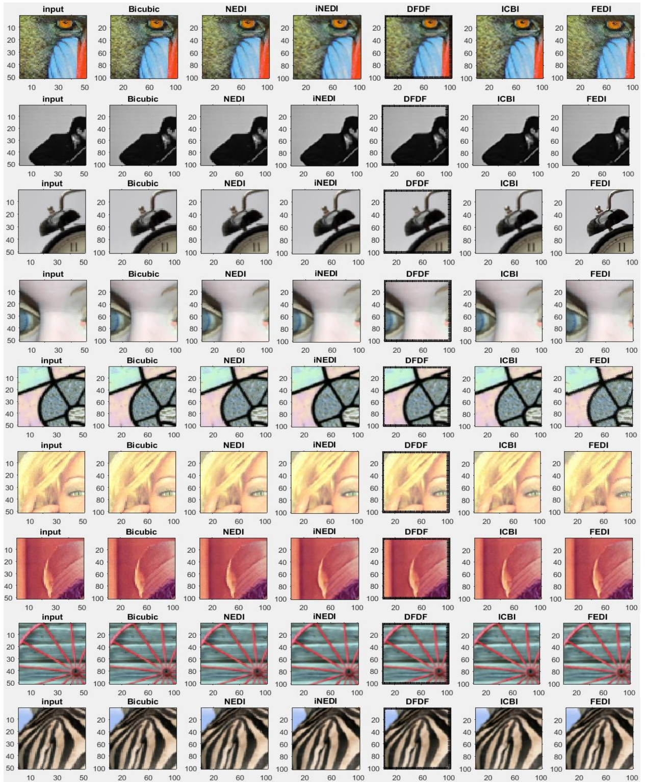
Fig. 5 Comparison of different edge directed image interpolations with 2x factor for some test images: From left to right: LR image, Bicubic, NEDI, iNEDI, DFDF, ICBI and proposed FEDI.
