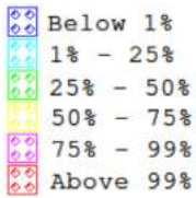
Figure 9. Colors and their respective ranges for heat maps. Defects inserted into dark blue cells led to error events in a circuit in less than 1% of the simulations, i.e. for every 100 defects inserted into the cell, no more than one of them resulted in an error event. Defects inserted into light blue colored cells led in 1-25% of all simulations to an error. Analogous reasoning may be applied to light green, yellow and pink colored cells complying with their respective percentage ranges indicated in the illustration. Defects inserted into red colored cells led in more than 99% of the simulations to an error.
