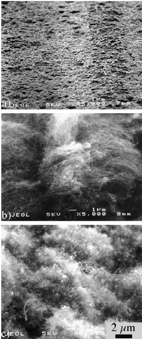
Fig. 1. SEM micrographs of CNTs grown at temperatures of (a) 600, (b) 625, and (c) 650 °C with 120 mM of iron nitrate during 65 min. The growth has been terminated by direct pumping. Micrographs a–c have been taken at the same magnification.
